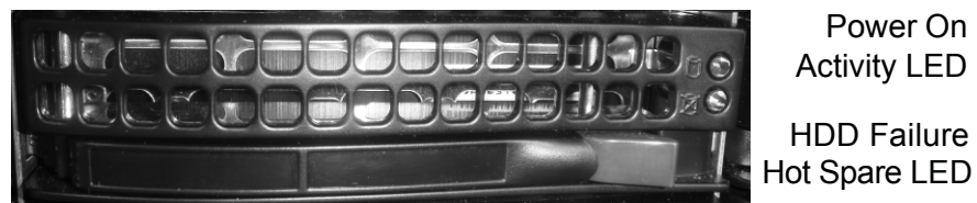
Figure 57. E12 SAS HDD LED Indicators
