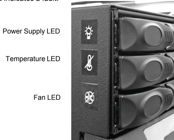
Figure 55. A12 SMS LED Indicators
